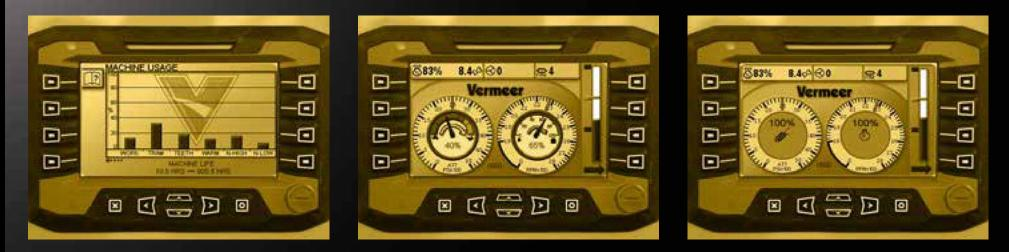
SmartTEC Performance Software assists operators with adjustments to machine controls to improve efficiency and tracks the productivity of the machine. Performance history is recorded, including individual operator history, for analysis by the machine owner or fleet manager. SmartTEC screens also offer a cleaner display, showing only what the operator needs to improve control and production.
